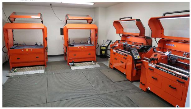
Most equipment techs would agree that a dedicated room for reel grinding is a must-have in a modern maintenance facility.
